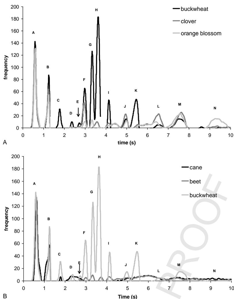
Fig. 1. Chromatograms of (A): buckwheat, clover, and orange blossom honey and (B): buckwheat honey, beet, and cane invert sugar. Letters indicate peaks considered for the PCA analysis.
