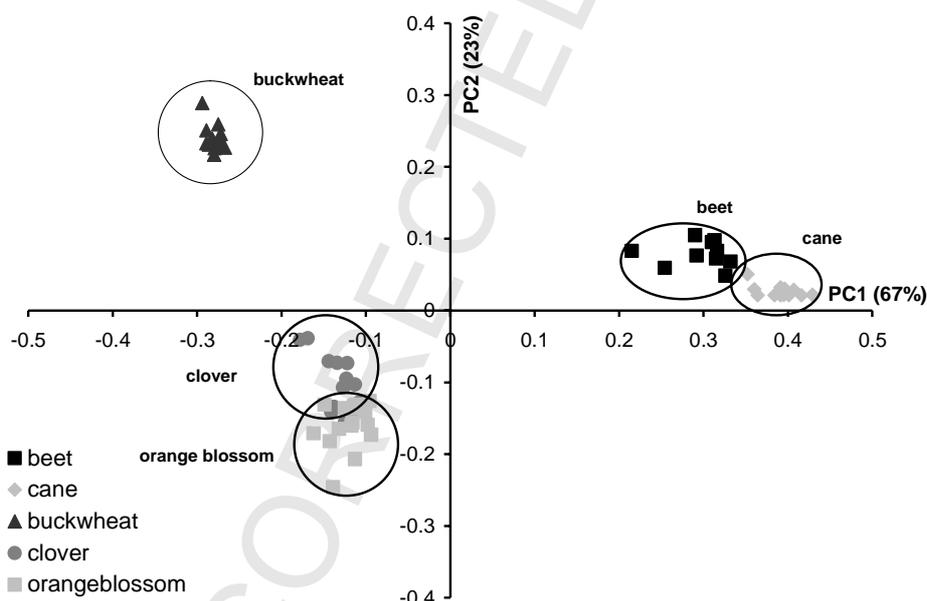
Fig. 4. PCA score plot of buckwheat honey, clover honey, orange blossom honey, beet invert sugar, and cane invert sugar, based on zNose<sup>TM</sup> chromatograms.
